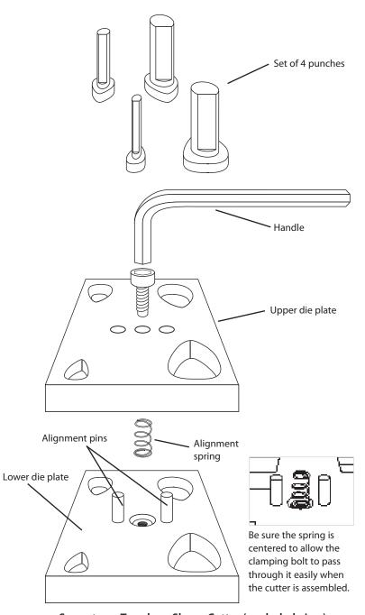
Swanstrom Teardrop-Shape Cutter (exploded view)
